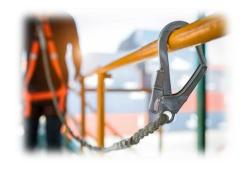
The worker must wear a safety belt of the parachutist type in activities above 2.00 meters in height in structures connected to the stand and with a risk of falling.
